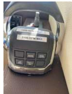
CAUTION SHOULD BE TAKEN: the THROTTLE/GEARSHIFT is SENSITIVE!! Go Easy. It only takes a slight nudge to put it in gear and initiate idle speed. Since it is electronic and not manually moving a cable, force is NOT NEEDED to make adjustments in speed, especially from neutral.
