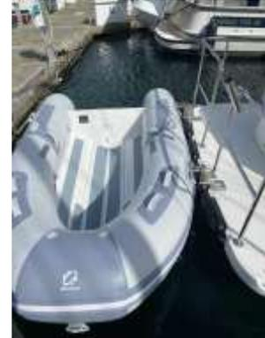
To deploy the dinghy, attach a raising / lowering line to the D-ring located on the starboard pontoon and tie it off to the boat. Then, detach the two STANDOFF BARS from the dinghy and transom and set them in the cockpit - to be stowed in the port lazarette. Lower the dinghy with the line, noting that the dinghy gets heavier as it nears the water. Detach the dinghy from the two Weaver brackets on the swim step. Reverse the process when stowing the dinghy for travel.
